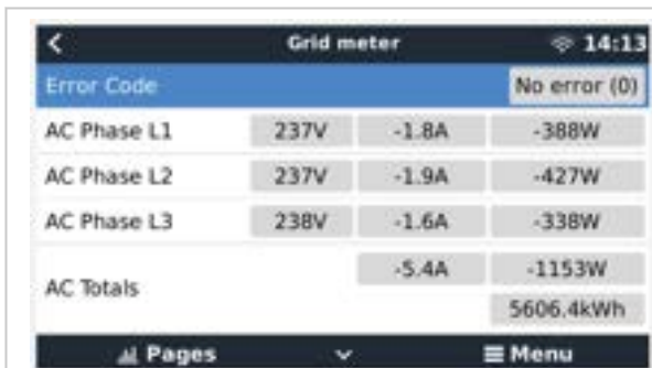
Detailed overview page of a 3-phase Grid meter
