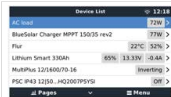
Energy meter set to measure AC loads on the AC output of the inverter/charger
