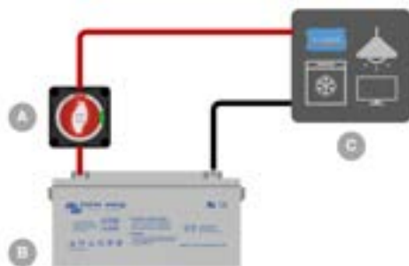
Battery Switch used to disconnect the house system from the house battery. Use to preserve battery charge, system maintenance or in an emergency.
